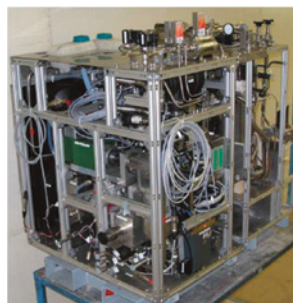
Figure 4 – Technology Platform 2: Fuel cell APU laboratory prototype during assembly.
